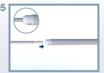
Mount the assembled fibre rod kit to the top of the top bracket.
