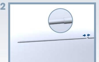
Assemble the two lower poles by inserting the upper pole into the plastic sleeve of the lower pole.
