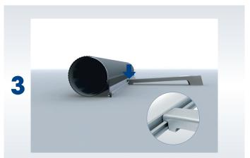
Attach the stabilizing foot to the lower panel profile.
