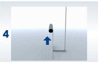
Take hold of the graphic panel and roll up. Place the supporting rod into circle cap on the stabilizing foot.
